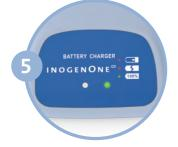
When the green light illuminates, the battery is fully charged\*.
